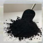
FeSfix : iron oxide based on one third FeO and two thirds Fe<sub>2</sub>O<sub>3</sub> with 50% iron (Fe) and natural trace elements.
