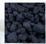
Metalox : a metal oxide based filter medium that reacts with H<sub>2</sub>S in the gas phase.
